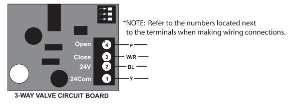
Figure 33 – 3-Way Valve Cover Connection Diagram
